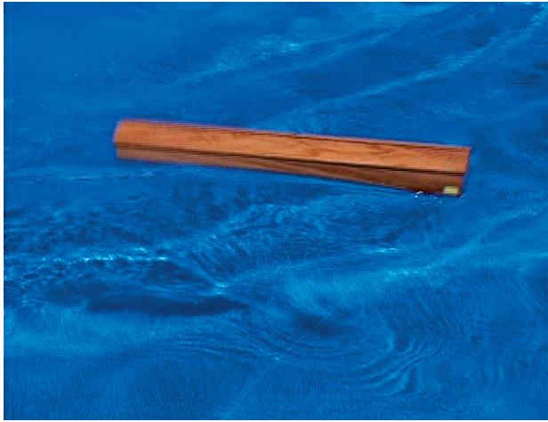
Figure 6. Free standing lightweight 1/200th scale ark model before waves. The marker on the lower right of the ark is a 1 inch marker. The weight of the vessel was 1.11 lbs. The depth from the bottom of the boat to the water line was 0.5 inches.
