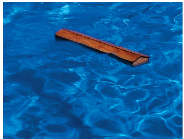
Figure 9. 1/200th scale ark model showing the baseline for the heavier weight model. The weight of the vessel with the extra water simulating food, animals, etc. was 7.82 lbs. The depth from the bottom of the boat to the water line was 1.75 inches.
